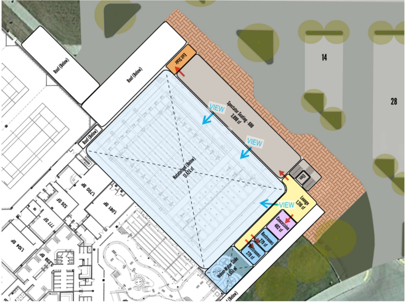
Figure 34: Indoor Aquatic Facility Concept – Mezzanine-Level Plan
